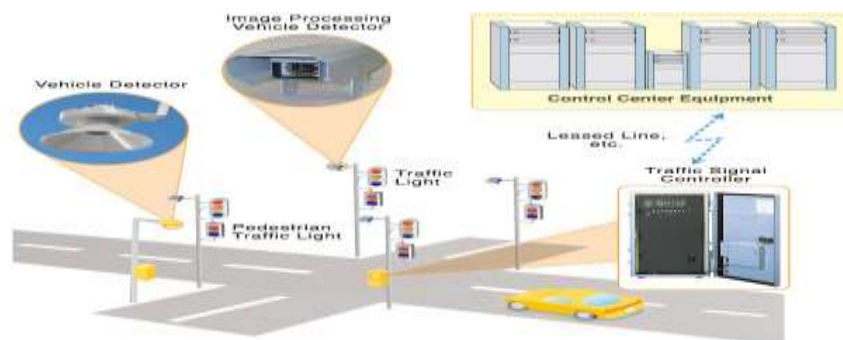
Figure 2: Smart Traffic Signal Control System Architecture
